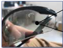
Heavy metal projectile that struck the safety glasses in the accident
