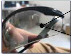
Heavy metal projectile that struck the safety glasses in the accident
